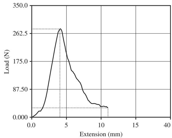
Fig. (10): Force/deformation curve of He-Ne photostimulated tendons group (A).
